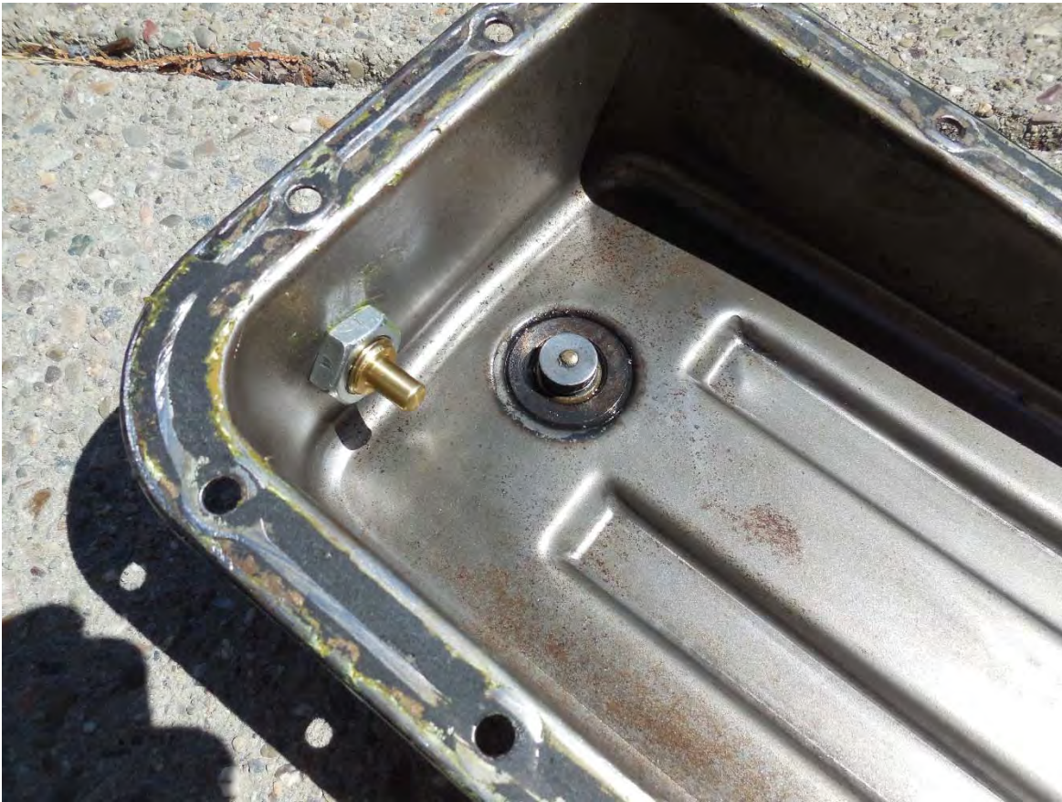
Mounting temp sensor in oil pan
