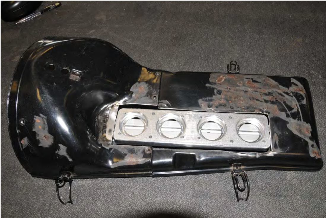
Modifying the air shroud opening to accommodate the manifold
