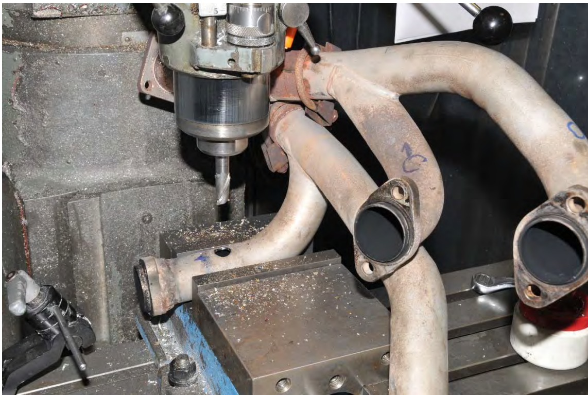
Machining bung holes in each header pipe to run four narrow-band O2 sensors
