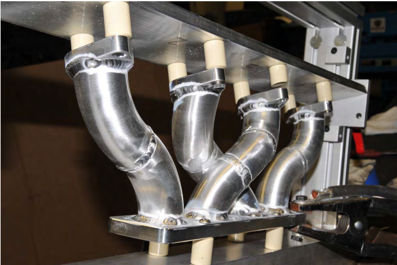
Fabricating intake manifold in special fixture
